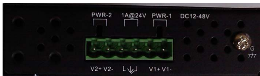
IES-2042PA power connection
